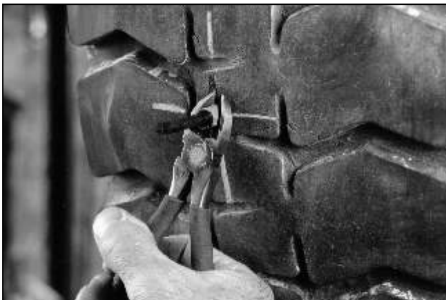
29 Cut the stem off on the outside of the tire 1/8" (3mm) above the tire's surface.
