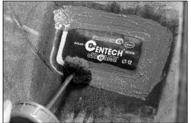
28 To cover over-buffed areas in tubeless tires, apply Security Coat to the outer edge of the repair unit and over-buffed areas. *If tube type, cover the repair with Tire Talc to prevent the repair from vulcanizing to the tube.
