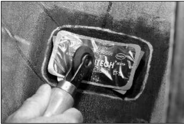
25 Stitch the repair unit down from the center out.
